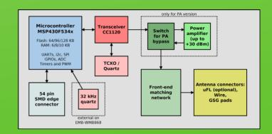
The stack already deals automatically the strict timings aspects imposed by the standards for synchronized transmissions in order to save as much power as possible. The module also provides firmware update functionalities as well as CRC and address check/insert for every packet. Multihop networks are also feasible.
