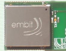
**EMB-ZRF231PA** is a 2.4 GHz OEM wireless module targeting low-power RF applications. The module is a simple and cost effective solution that provides IEEE 802.15.4 / ZigBee® wireless connectivity and multi-hop networking.
