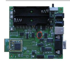
2x3 ways 2,54 mm pitch header male connector, for interfacing to the SPI lines.
