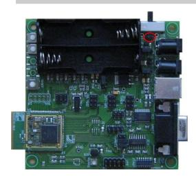
Header connector for powering the RF module.
