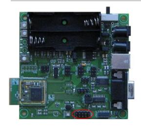
2x5 ways 2,54 mm pitch header male connector, for interfacing to the analog lines (where available).
