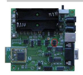
2x3 ways 2,54 mm pitch header male connector, for interfacing to the timer lines. Pin 1 is bottom right (in figure).
