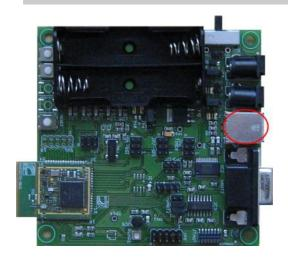
Type B USB connector (2.0 full-speed compatible) which allows accessing from a PC to the UART1 of the module through a virtual serial port over USB (FTDI FT232R USB-to-Serial UART converter). The UART to USB conversion implements a full UART with hardware flow control (TX, RX, RTS, CTS). Furthermore the USB port can be used to power the board.
