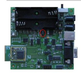
The highlighted header is used to select the power source that will be supplied to the module. If the jumper is mounted on the higher position (3-2 as seen in the picture), the module voltage supply will come from the board voltage supply. If the jumper is mounted on the lower position (1-2), the module will be powered directly from the external source present in the unfiltered power connector (X4).
