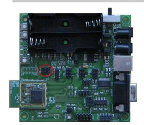
2x3 ways 2,54 mm pitch header male connector, for interfacing to Atmel's PDI programming interface.
