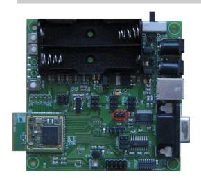
3 ways 2,54 mm pitch header male connector, for interfacing to the I2C bus. Pin 1 is left (in figure).
