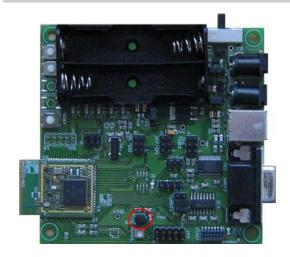
An analog temperature sensor (National Semiconductor LM61BIZ) is installed on the board and connected to the ADC6 line. The output of the sensor is 10 mV /  $^{\circ}$ C with an offset of +600 mV.
