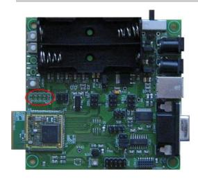
2x5 ways 2,54 mm pitch header male connector, for interfacing to the digital lines used on the board for switches and LEDs.
