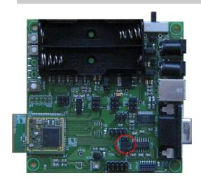
With this header the signals coming from UART2 can be connected to the UART to RS232 converter (with two jumpers). If the jumpers are removed, the UART2 port can be connected with an external system. The two pins on top are connected to ground, the second row of pins are the module RX line (on the left) and the converter TX line (on the right). The last row of pins (those on the bottom) are the module TX line (on the left) and the converter RX line (on the right).
