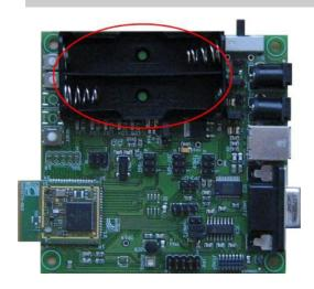
Slot for 2 AA alkaline batteries (1,5 V). The batteries must be connected with the proper orientation.
