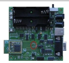
The board features soldering pads to install an external i2c memory in order to test the i2c bus or for firmware swap.
