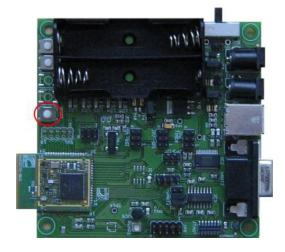
The hardware reset of the module can be forced by pressing the SW5 button. The switch signal is kept high by a 10 kOhm pull-up resistor and the signal is routed to the RESET# pin on the module (pin 51) through a 1 kOhm series resistor. By pressing SW5 the RESET# line is grounded (through this 1 kOhm resistor).
