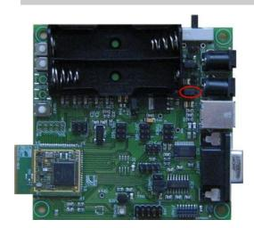
The highlighted header is used to select the power source that will be supplied to the board. If the jumper is mounted on the right (3-2), the board power will come from the batteries. If the jumper is mounted on the left (1-2 as seen in the picture), the board power will come from the voltage regulator.
