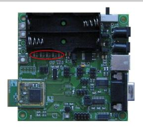
The 4 leds mounted on the board are connected to 4 GPIO lines as follows:
