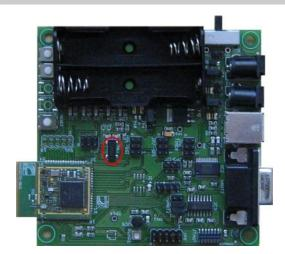
A 32.768 kHz crystal is installed on the board for obtaining an accurate RTC. The component (ABS25 Abracon Corporation family) is connected to the XTAL\_IN (pin 49) and XTAL\_OUT (pin 50) lines of the module.
