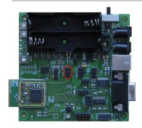
2x3 ways 2,54 mm pitch header male connector, for interfacing to the SSI lines (where available).
