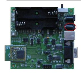
Coaxial male connector for powering the board. Specifications:
