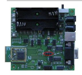
The UART1 serial port of the RF module can be interfaced through the USB connector or with a header. The UART1 signals from the module are connected directly to this header and then, with some 1.5 kOhm resistors for those signals driven by the USB to UART converter, to the converter itself. If the user needs to use the UART it can force the status of the pins through this header.
