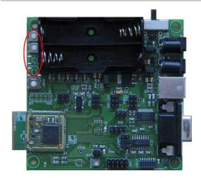
The 4 push-button on the board (some might not be mounted) are connected to 4 GPIOs that can handle interrupts. By pushing a button, the corresponding line is grounded.
