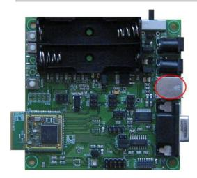
The board circuitry can be powered directly from a USB bus by plugging the USB cable to the USB connector (USB Type B).
