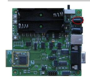
Coaxial male connector for powering the RF module. With this connector it is possible to power the RF module itself bypassing the whole board to measure current consumption, for example. There is no regulation stage here, the power provided is delivered directly to the module. Specifications:
