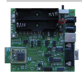
The highlighted header is used to select the external power source to be filtered. If the jumper is mounted on the right (1-2), the voltage regulator will be powered by the external supply connected to the filtered power connector. If the jumper is mounted on the left (2-3 as seen in the picture), the voltage regulator source will be the USB connector.
