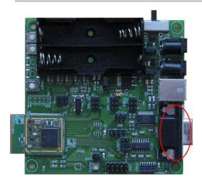
DSUB 9 ways female connector for interfacing to RS-232 buses. This connector allows the connection from module to host over the UART2 serial port. The RS232 line is not equipped for hardware flow control.
