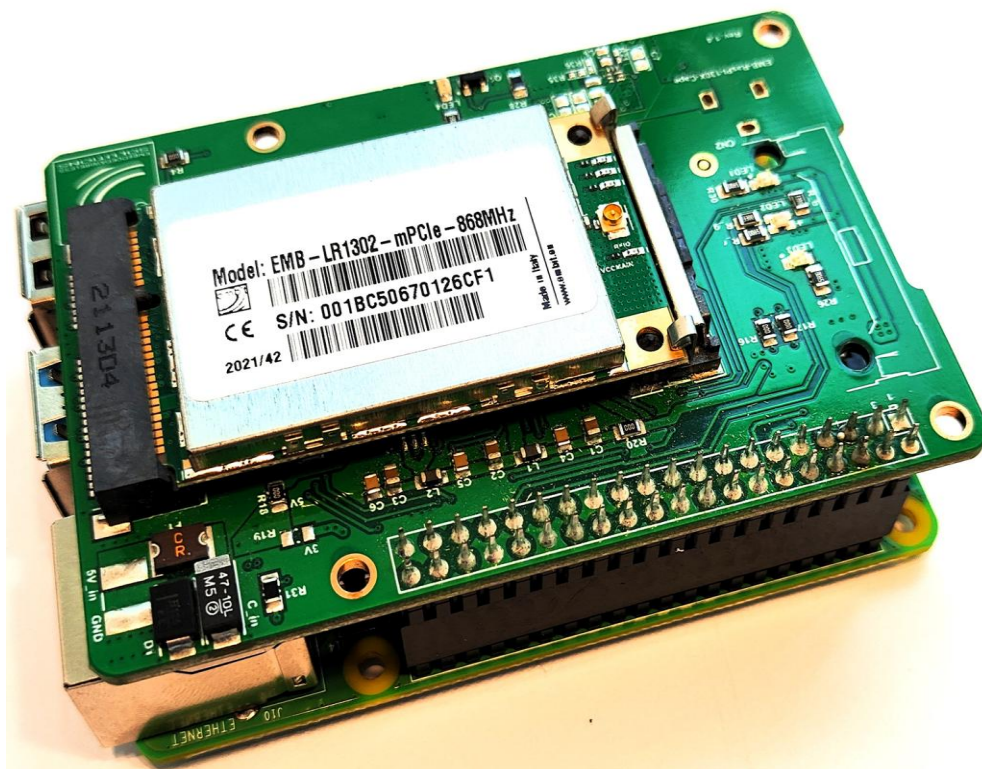
Figure 3. LoRa gateway with EMB-1302-mPCIe + EMB-RasPI-130x-Cape + Raspberry Pi Board
