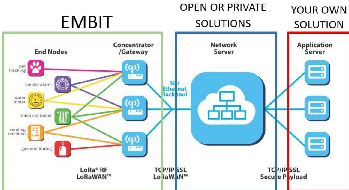
Figure 4 LoRa® Network Architecture
