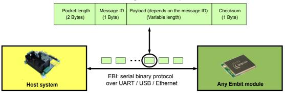
(Embit module is configured as "flexible modem" and is loaded with the EBI firmware)
