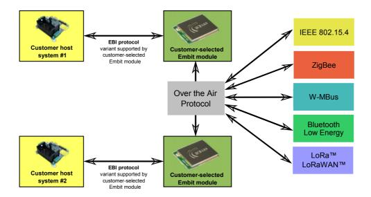
In particular, the EBI protocol supports several commands that *abstract* the features of over-the-air protocols. For this reason, the majority of EBI commands are common to all Embit modules; a portion of the EBI commands are available only on some specific Embit wireless modules (see Section 2.4). Due to this, EBI documentation is divided in several documents:
