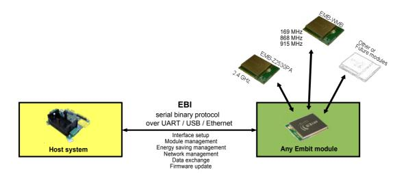
A firmware application implementing the EBI protocol is available for all Embit modules, so that any Embit wireless module can be employed as a "flexible modem" using simple AT-like commands. The EBI protocol also accounts for the fact that different Embit wireless modules support different over-the-air protocols (e.g., some of them support only Wireless M-Bus, others support both IEEE 802.15.4 and ZigBee, etc):
